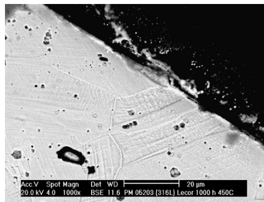
Fig. 4. AISI 316L specimens after 1000 h of exposure, LECOR.
